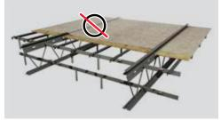
A sheet of polythene can be placed directly over the plywood in order to protect it and facilitate removal afterwards. The polythene should never cover the joist or the top chord. No materials whatsoever should cover the top chord so as not to impact the joist's composite action.
