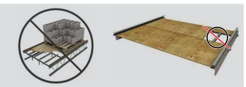
Do not overload the slab or joists during construction with materials such as palettes of cement blocks, dry stone walls, sand, etc.
