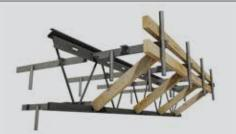
This system is applicable to cantilever slabs  $\leq$  1 ft.-2% in. (375 mm). For cantilever slabs > 1 ft.-2% in. (375 mm), the system must be stabilized; refer to the recommendations of the consulting engineer.
